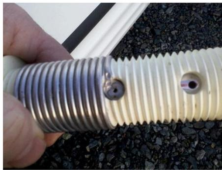
coils, you couldn’t help but notice a missing one inch piece of the aluminum wire on the larger coil, and on the small coil, it had melted away from the rivet. Inspection of its twin on the other half of the dipole, showed no damage at all and it was totally clean inside the tube.
