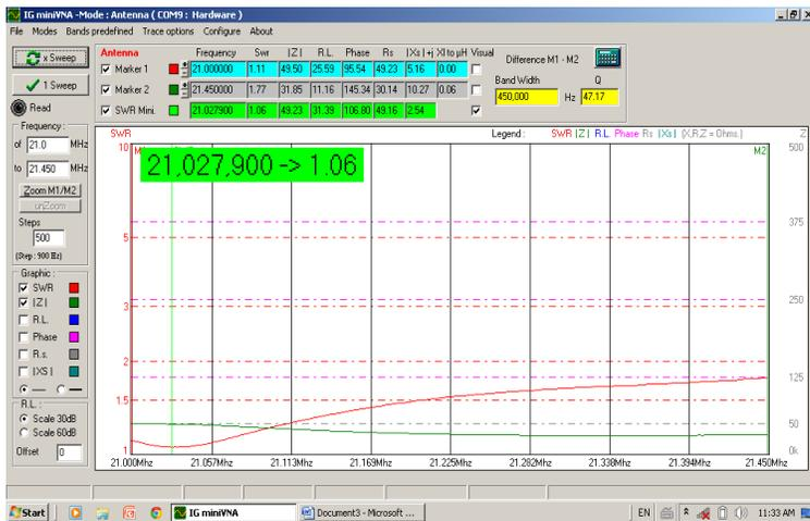
Next, the 15 metre band. As you can see, it was under 1.77:1 across the entire 21.0 to 21.450 MHz band. Interesting to see that it favoured the CW portion as well, with a resonant dip at 21.0279 and SWR of 1.06:1.
