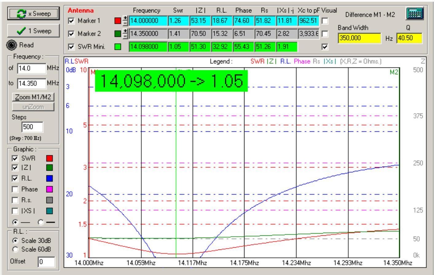
You can see the resonance has dropped considerably—down to 14.098 with a SWR of a respectable 1.05:1 [red line]. The return loss [blue line] is well below -30db which is what is expected with a low SWR. The green impedance line is good too, staying close to 52 ohms.
