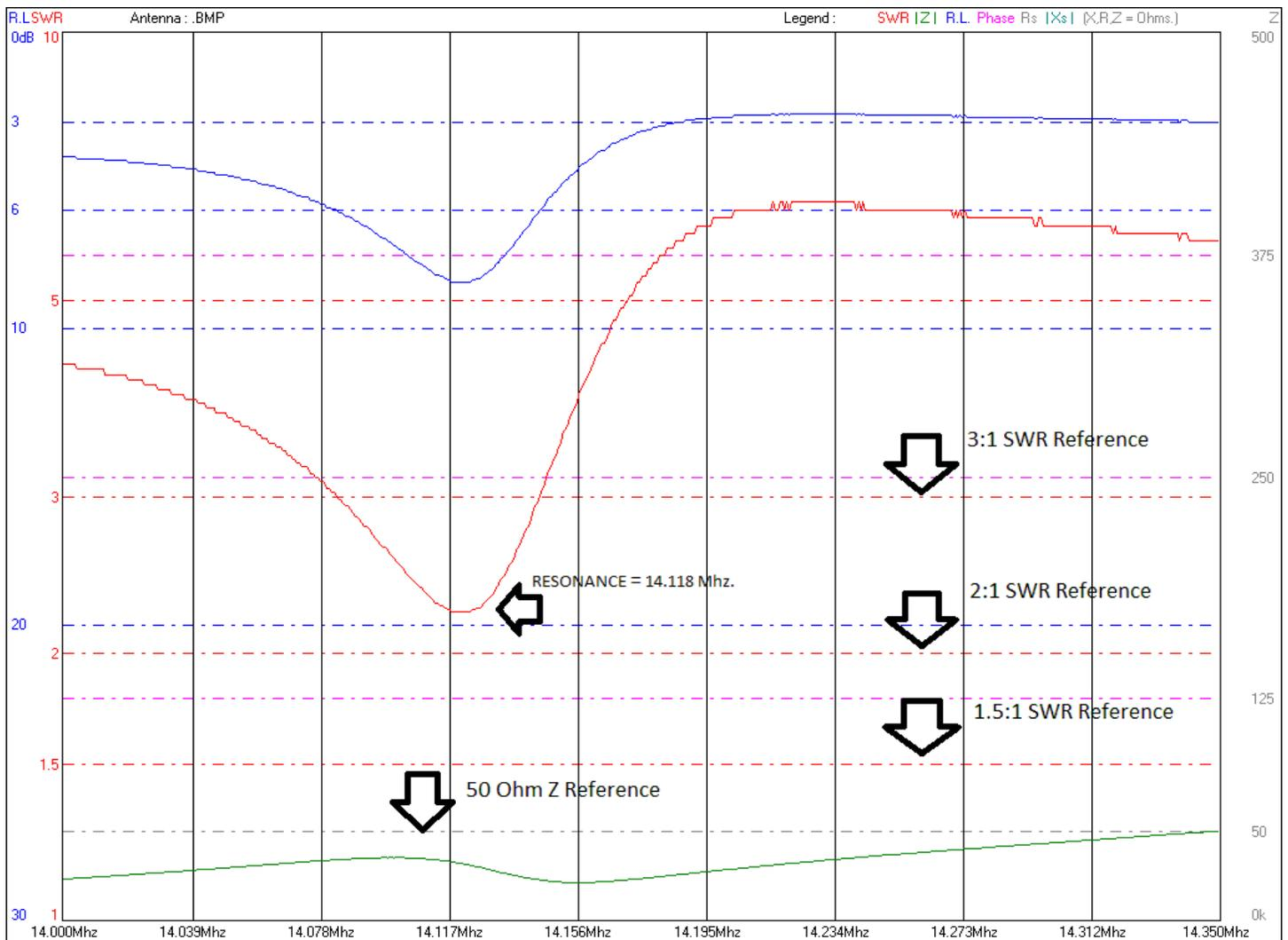
Above is a 14.0 to 14.350MHz. VNA scan. The blue line represents the Return Loss, which should be greater than -30db down, it's only -8db—dismal. The red line is the SWR and it's only below 3:1 between 14.080 to 14.140—not good. The Impedance line [green] shows that it's below 50 ohms—not what I was expecting. So something was wrong—I am reminded of items 1 to 4 on the previous page for the reason.
