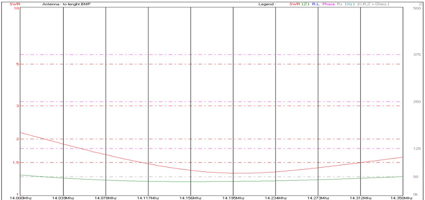
As you can see in the graph above, the 2:1 bandwidth expanded to 14.050 to 14.350, or basically 90% of the 20m band. Resonance was around 14.190 Mhz. and the Z [impedance] very close to 50 ohms, but more importantly almost flat across the band. So with just adding the reflector to the driven, we have a 3db gain 2el Yagi... Useable as is! Why? Because the gamma match needs the interaction of the parasitic element to work it's phasing magic.
